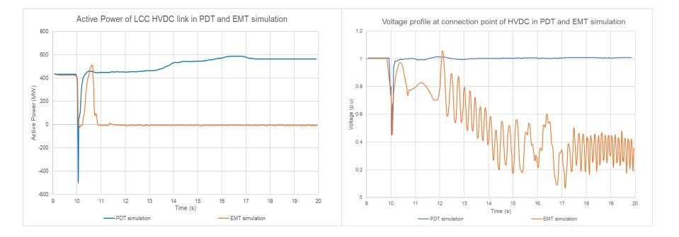
PDT model does not predict sustained commutation failure and subsequent disconnection of the HVDC link
