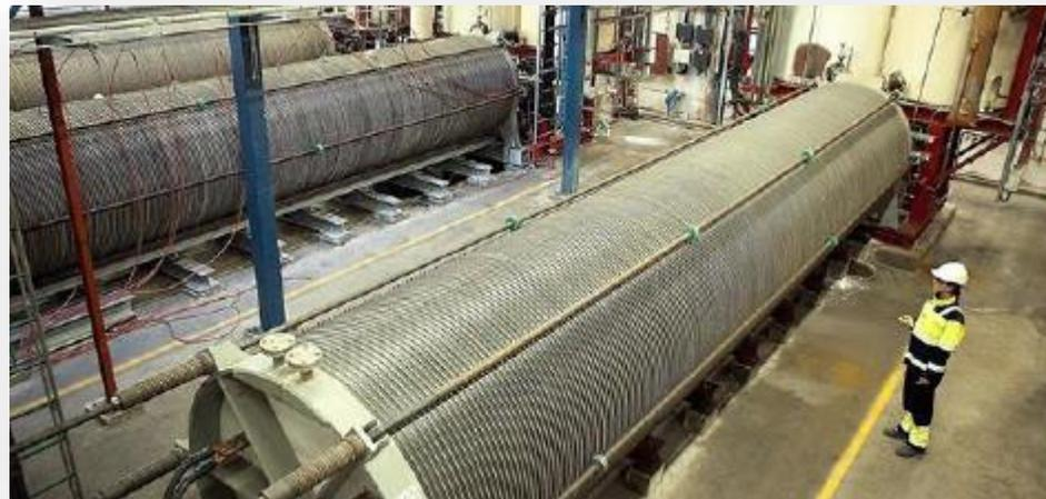
2.25 MW alkaline stack
