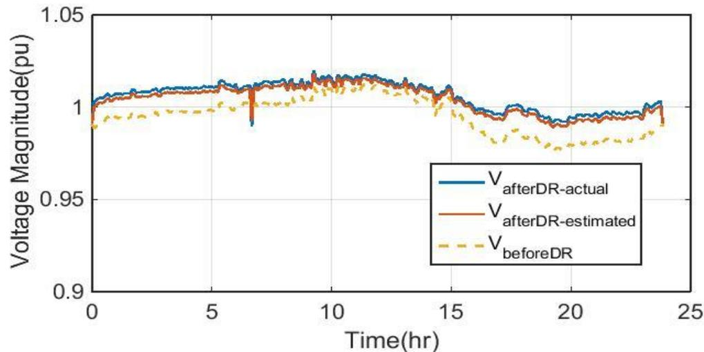
Voltage profiles at node 11 phase A
