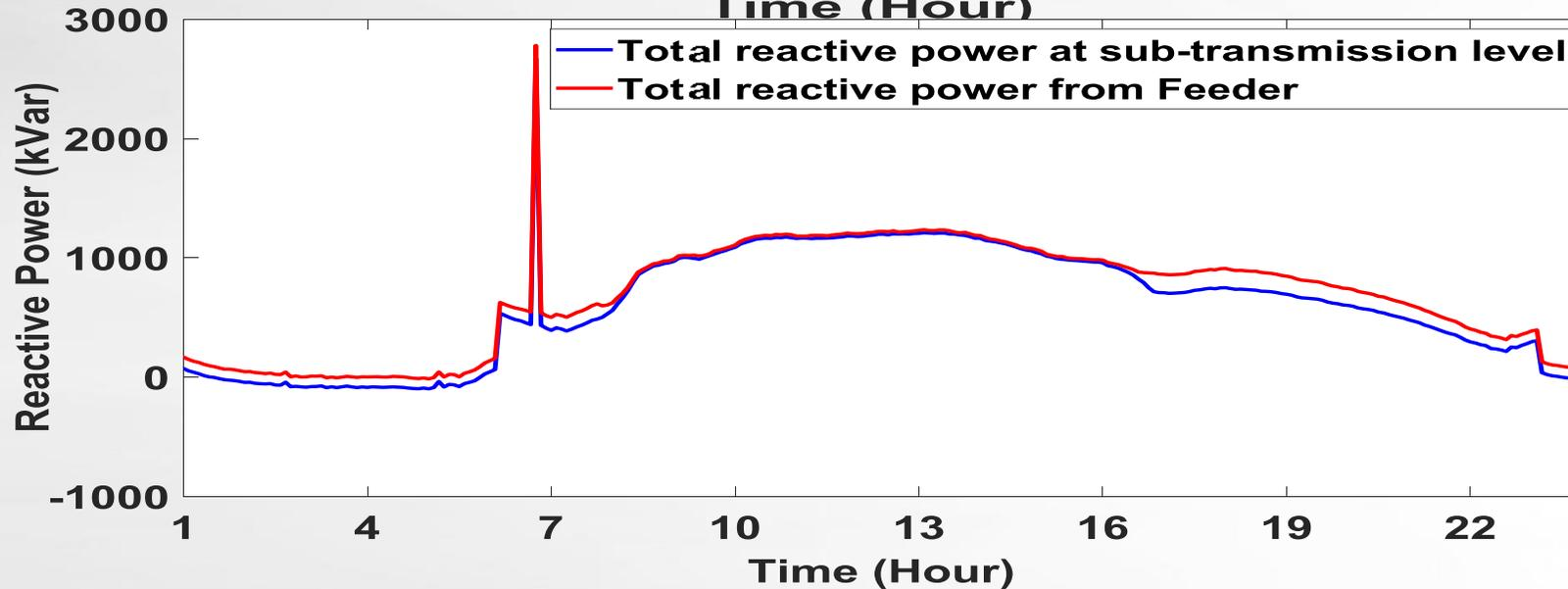
Distributed PV is able to meet reactive power requirements to support sub-transmission voltage.
