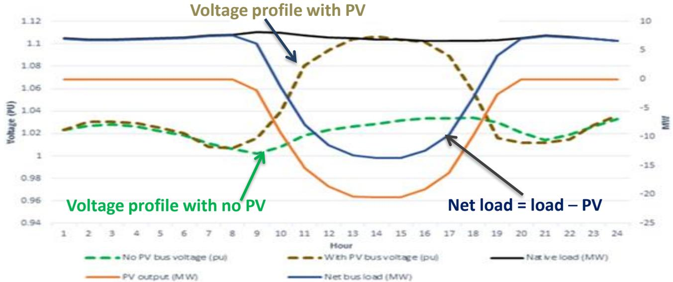
**Under low load condition and high PV penetration, there is a potential for over-voltage problems**
