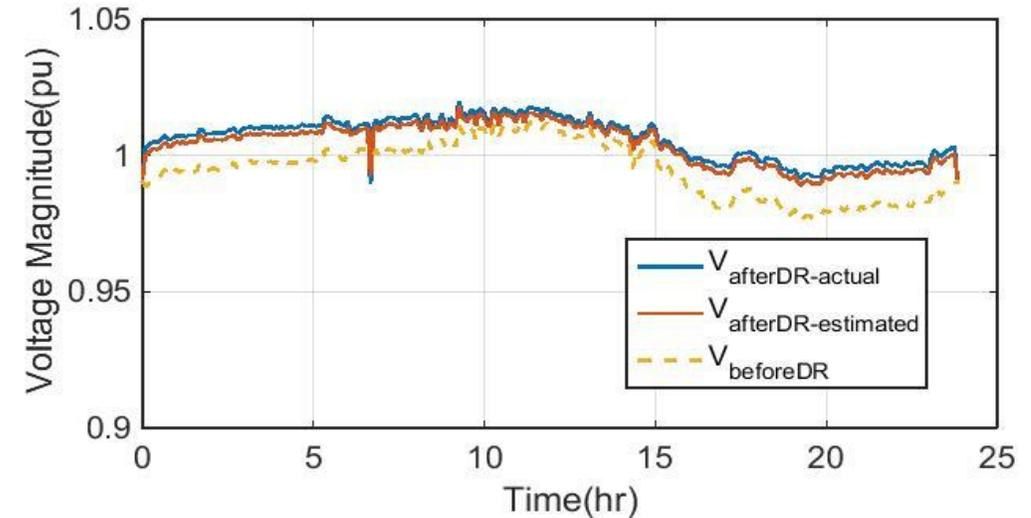
Voltage profiles at node 65 phase C
