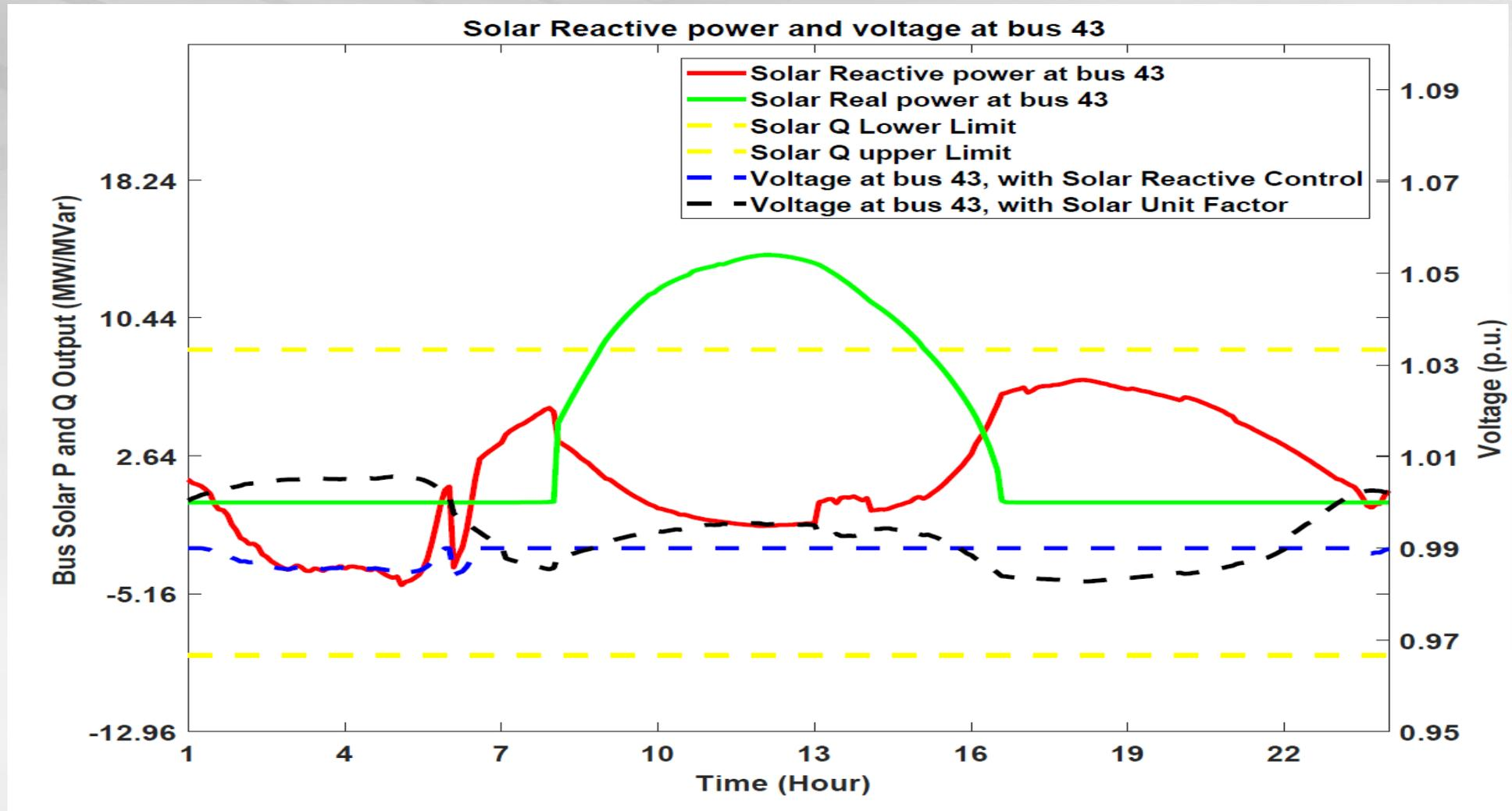
Aggregated reactive power from distributed PV (red line) is able to maintain the target substation voltage (blue dotted line).
