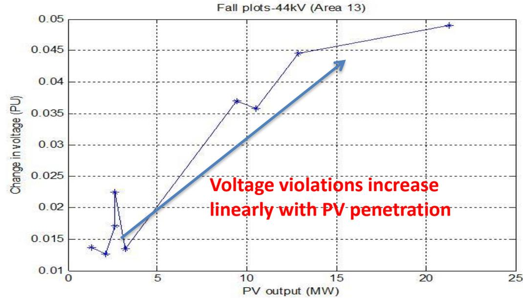
System voltage magnitudes increase almost proportionally when the PV outputs increase
