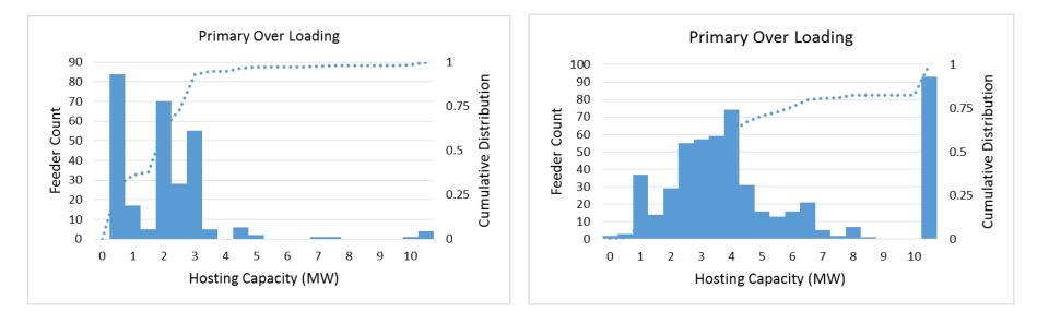
The hosting capacity is driven by the lowest rated three-phase conductor on the feeder. The hosting capacities elsewhere on the feeder can be considerably higher
