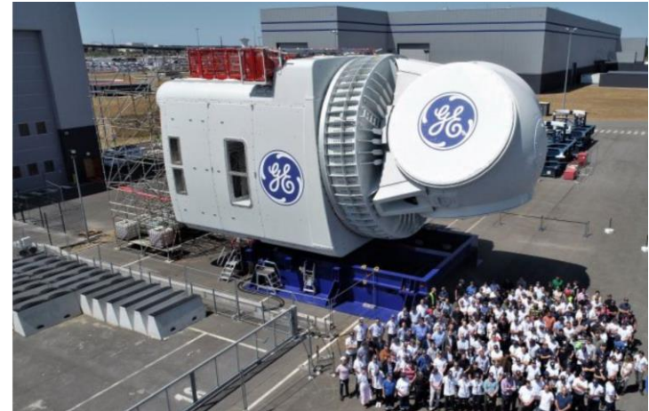
GE 12-MW Wind Turbine Nacelle – Haliade -X
