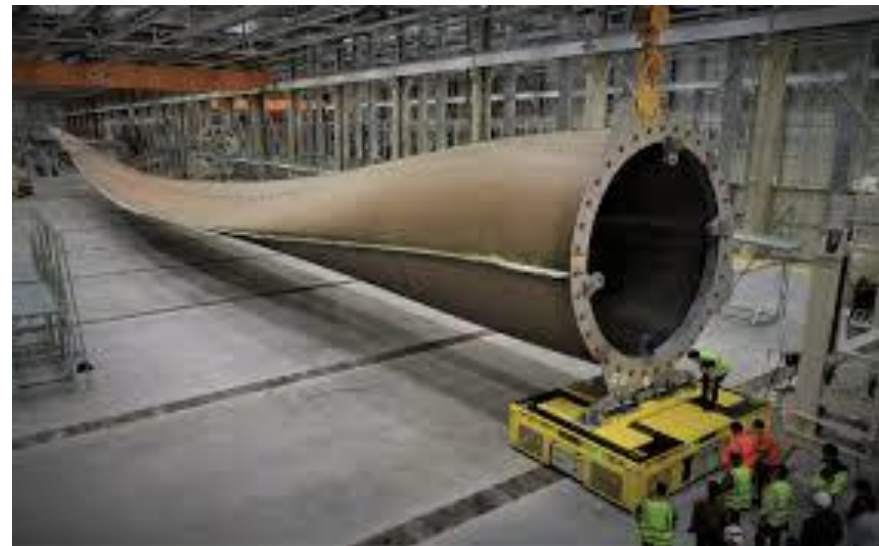
GE Haliade 12-MW 107-meter Blade Prototype – Longest Blade Ever Built
