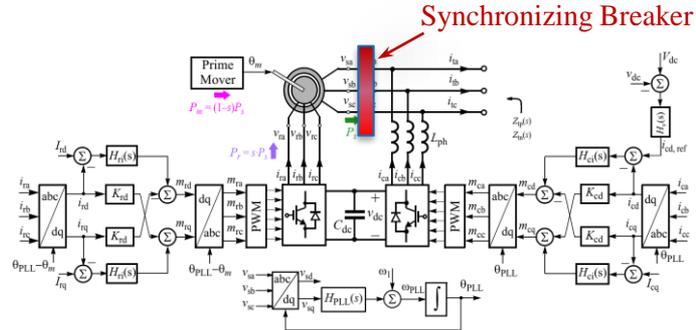
Fig. 1. Circuit and control diagram of a doubly-fed induction generator (DFIG).
