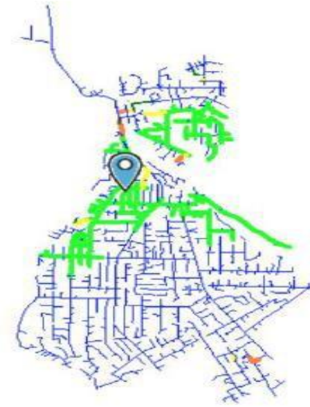
Peak 2034 COM Power Flow After Mitigation
