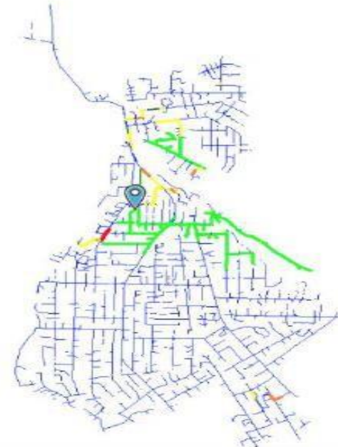
Peak 2034 RESI Power Flow After Mitigation
